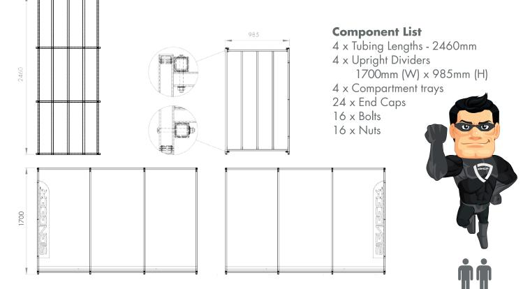
For ease of assembly, we recommend that you assemble the rack on its side. Once all fixings are tight and secure, secure the trays as shown in the image above.
