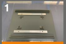
Prepare panel with channel, cut and drilled flat bar and M8 nuts, bolts and washers
